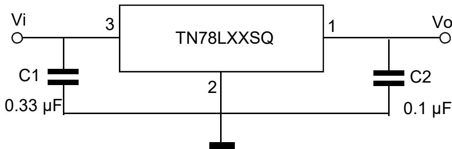
Note: Bypass capacitors are recommended for optimum stability and transient response and should be located as close as possible to the regulators.
