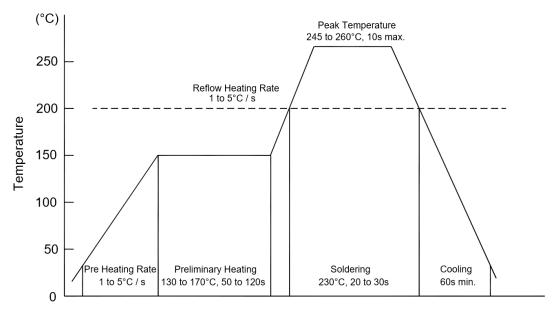
Recommended peak temperature is over 245 °C. If peak temperature is below 245 °C, you may adjust the following parameters:
