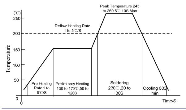
Recommended peak temperature is over 245° C. If peak temperature is below 245° C, you may adjust the following parameters:
